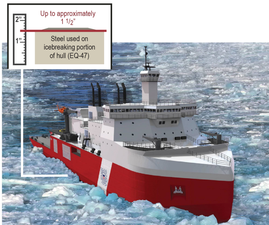
Figure 6: Polar Security Cutter's Hull Thickness along Icebelt
