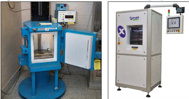
Figure 7: Irradiator with Radioactive Material (left) and Alternative Technology (right)
