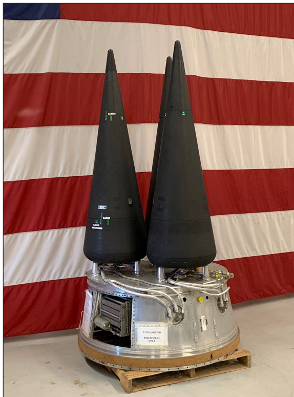
Figure 11: Mk12A Reentry Vehicle in a Multiple Independently Targetable Reentry Vehicle (MIRV) Configuration
