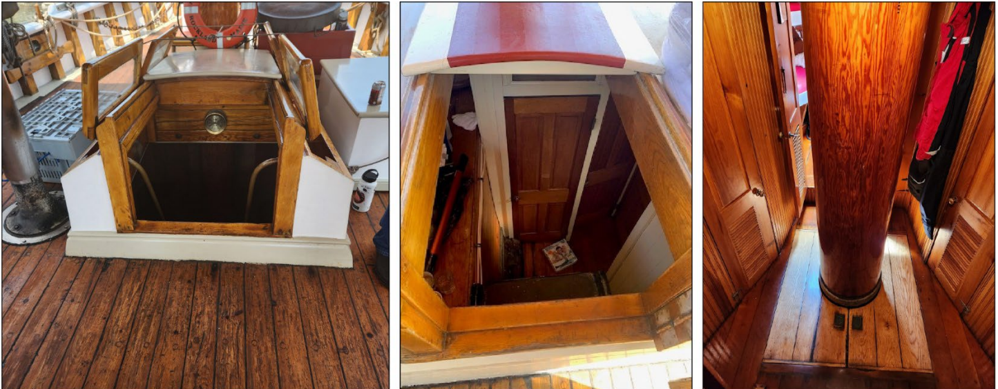
Figure 4: Examples of Means of Escape from Accommodation Spaces on Wood Sailing Vessels
