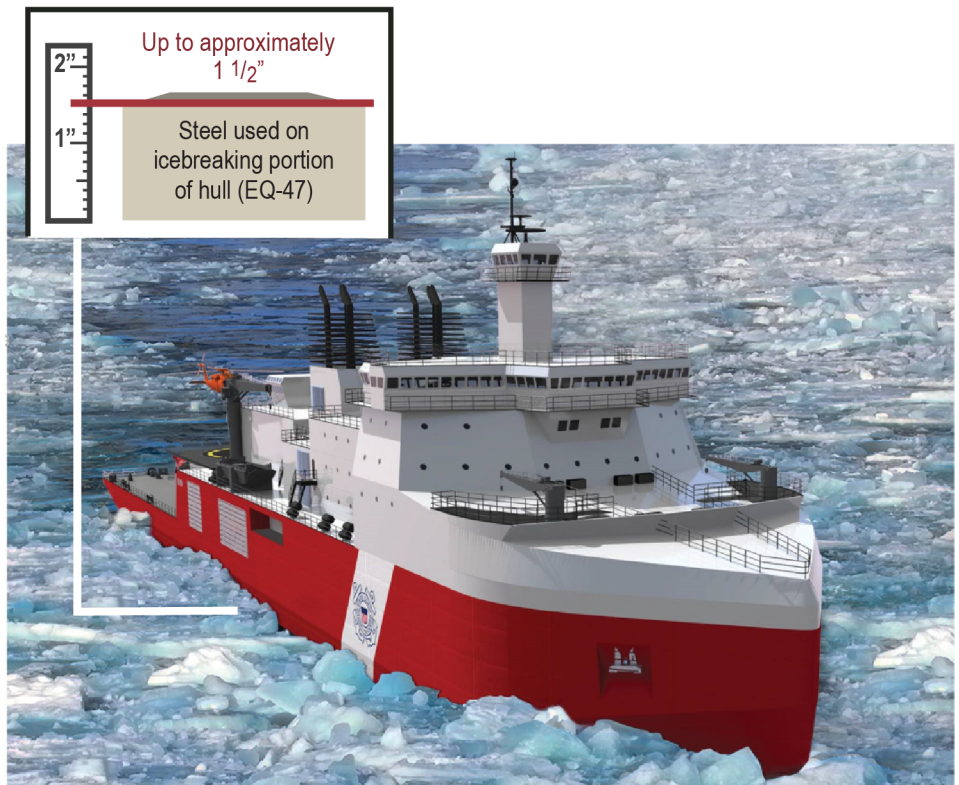
Figure 6: Polar Security Cutter's Hull Thickness along Icebelt
