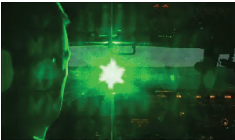
Figure 7: Example of the Effects of a Laser Pointer Aimed at an Aircraft Cockpit
