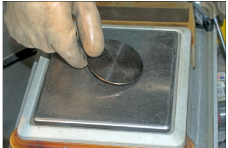
Inspecting and weighing plutonium metal sample
