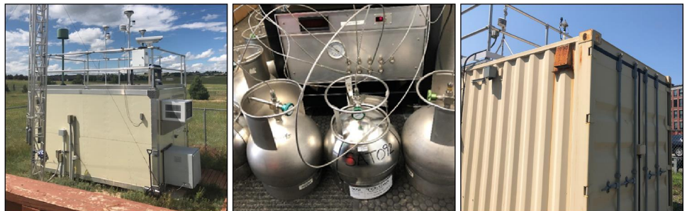
(Left to right) National Core network (NCore) monitoring site; canisters used to collect samples for measuring air toxics; near-road monitoring site.
