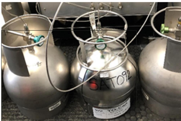
Figure 2: Example of Air Toxics Monitoring Equipment
