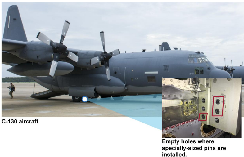
Figure 6: Benefits of Using Specially-Sized Pins on Shelf Brackets for C-130 Aircraft at Ogden Air Logistics Complex, Utah
