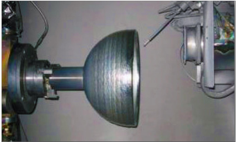
Figure 4: Additively Manufacturing a Satellite Propellant Tank Using Electron Beam Technology
