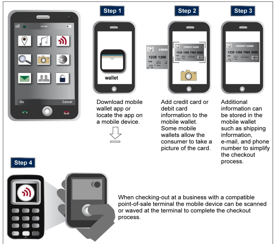
Figure 3: How Mobile Wallets Work in Stores
